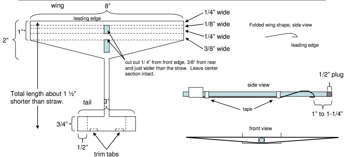
Below is a simpler glider pattern that can be cut from paper (enlarge so each glider pattern is 6" long, 5" wide). Folding the center section up and taping it forms a triangular fuselage beam that stiffens the paper enough to hold the wings straight. Use 1/2" of clay in the nose and let the straw protrude 1-1/4" from the front wing edge for balance.
