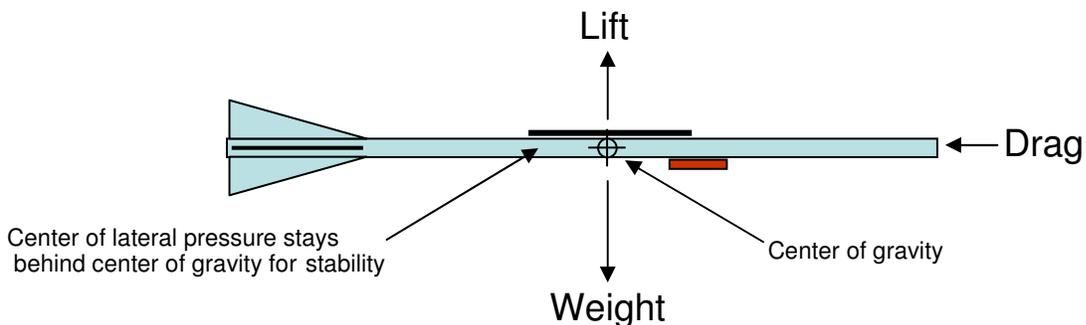
This activity differs from making and flying paper airplanes in that the launcher allows precise comparison between designs because the launch angle and force is controllable and repeatable. Winged rockets should be launched at a low angle to allow them to glide rather than just follow a ballistic trajectory. Launching at angles above about 30 degrees gives results that will differ little from a basic straw rocket.
