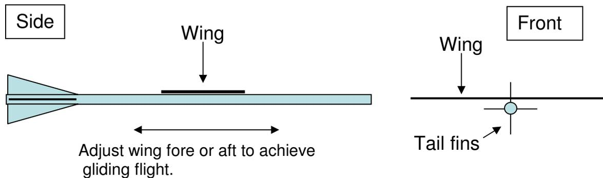
You can also make the above adjustment by taping a small ballast weight ( ½ “ of thick wire or a paperclip) to the bottom of the rocket tube. Move the weight aft if the rocket noses down. Move it forward if the rocket noses up too much.
